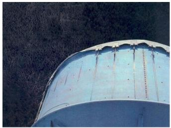
Figure 4: Missing Radome Mounts
